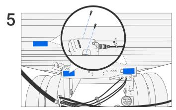
Select the desired mounting location. For best GPS and cellular connectivity results, mount as close to the edge of the trailer as possible and consider the motion of the moving parts that may damage the device or the cables. If possible, test the device in the desired mounting location before installation.
