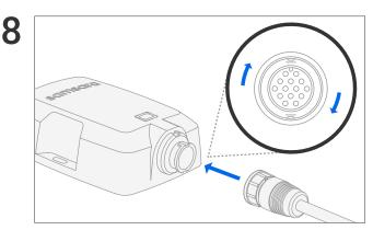
Plug the cable into the AG and twist to lock.
