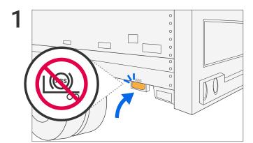
Before you attempt installation of the AG on your trailer, ensure that the ABS is in good working order: after trailer startup, the ABS light comes on for 3 to 5 seconds during startup before it powers off. Any other outcome may indicate a problem with the trailer ABS system. Turn off the power to the trailer.
