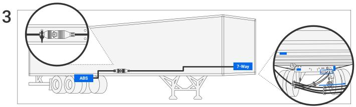
Locate and disconnect the 5-pin ABS Weather-Pack ("TTMA") connector on your trailer (typically located near the rear axle). To locate the connector, trace the wire harness from the ABS unit.
