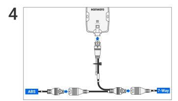
Connect the trailer's 5-pin connection to the Samsara cable using both of the two connectors you've just disconnected.
