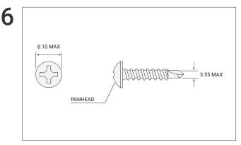
Mount the AG with the two provided screws or with screws less than or equal to #6 size, with a maximum torque of 1.4 Nm (12.4 lbf-in).
