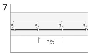
Secure the wire harness every 30 to 50 cm using cable ties while ensuring that the cables are free from sharp edges, bending load, or tension.
