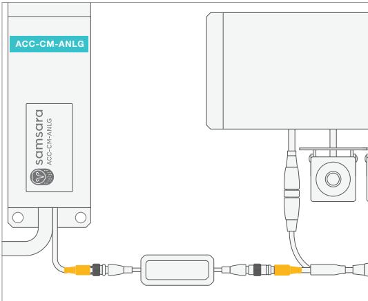
**EN** Connect ACC-CM-ANLG (with isolator attached) to video output.
