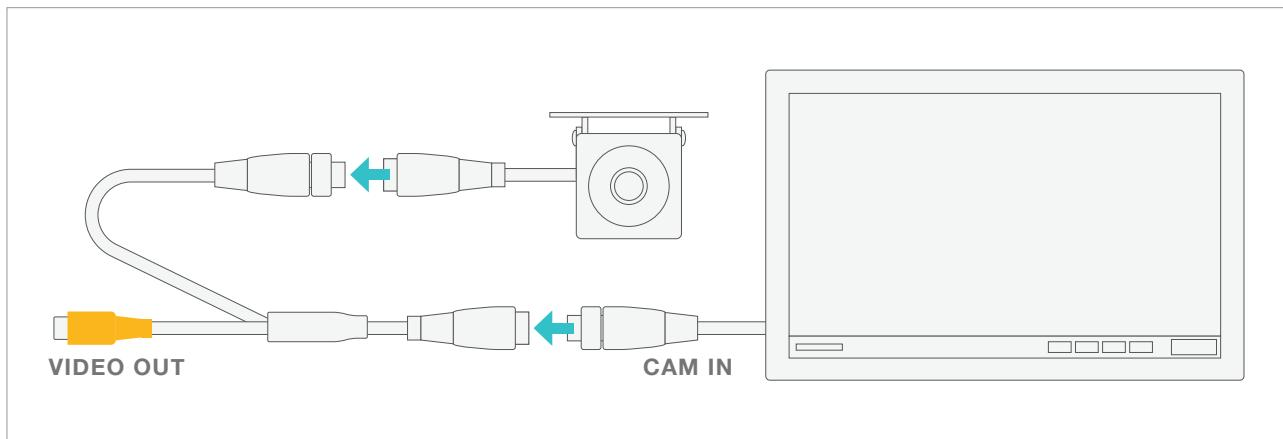
**EN** If display/DVR has camera input and video output, connect camera directly to camera input.
