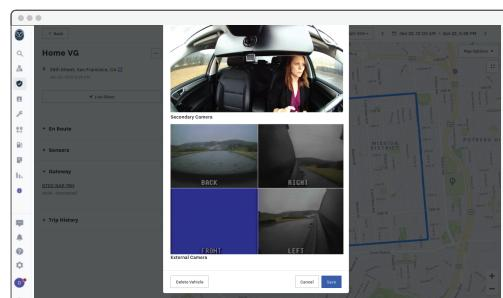
**EN** From the "Check Dash Cam Installation" feature, scroll through and verify that all camera images appear normally. Video feed from third party camera should appear in the section labelled "External Camera"
