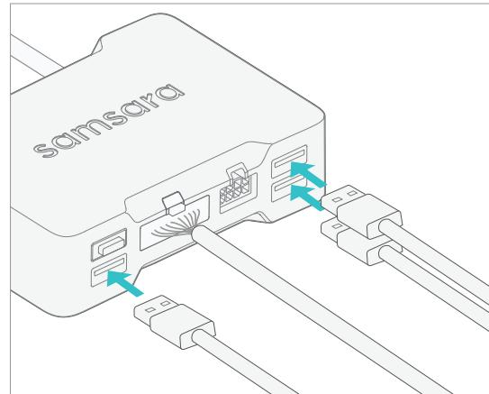
**EN** Connect USB cables from the CM dashcam and ACC-CM-ANLG to the ACC-BDHE diagnostics hub.
